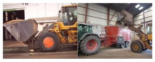
Figure 6: Manual mixing of raw materials
