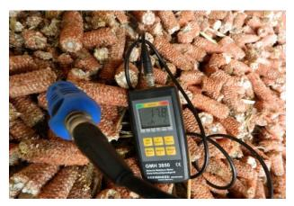
Figure 17. Moisture checking in raw material
