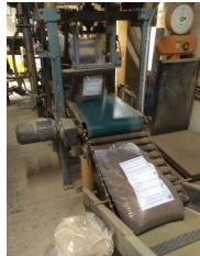
Figure 15: Sealing machine for bags
