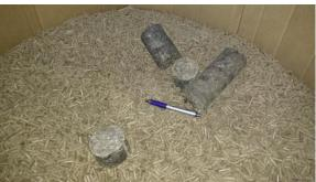
Figure 6: pellet and briquettes from vineyard pruning, produced by Costruzioni Nazzareno
